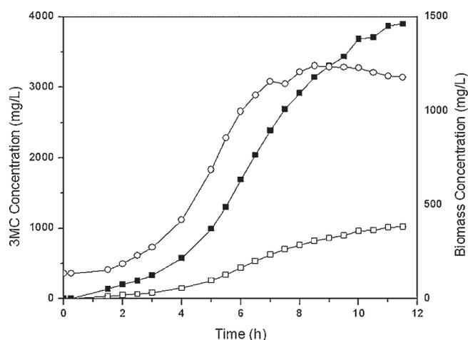
**Figure 2.** Bioproduction of 3MC in a two-phase bioreactor employing HYTREL™ polymer beads, in a 10% (w/w) phase ratio, as the immiscible phase. Circles represent biomass, hollow squares represent aqueous 3MC concentrations, and solid squares represent the total 3MC concentration in the system.
