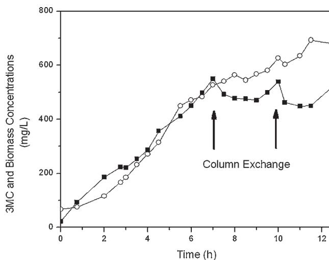
**Figure 4.** Bioproduction of 3MC in a continuous solid–liquid bioreactor. Circulation of medium through column was initiated at  $t = 2.75$  h. Column exchanges occurred at  $t = 7$  h and  $t = 10$  h. The biotransformation was terminated at  $t = 12.5$  h at which time aqueous 3MC concentrations reached 500 mg/L. Circles represent biomass and the squares represent aqueous 3MC concentration.
