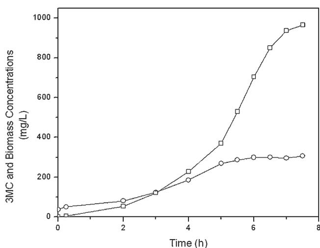
**Figure 1.** Single-phase bioproduction of 3MC. Squares represent 3MC concentration and circles represent biomass.
