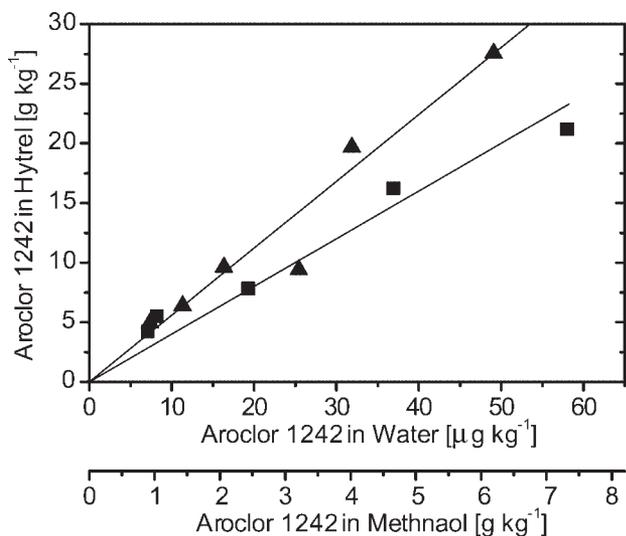
**Figure 2.** Partitioning of Aroclor<sup>®</sup> 1242 between methanol and Hytrel<sup>™</sup> (triangles) and between water and Hytrel<sup>™</sup> (squares).
