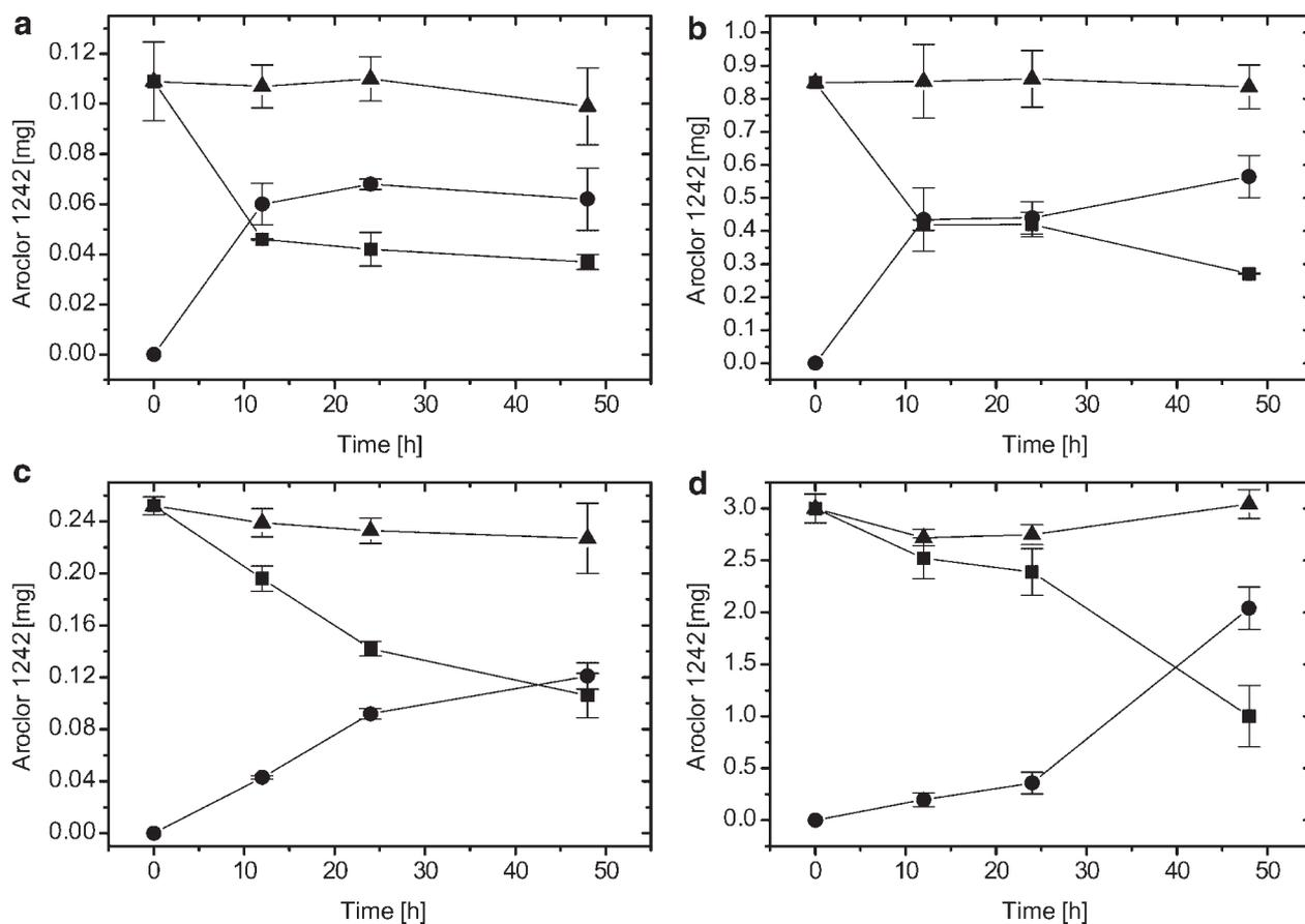
**Figure 3.** Time course of PCB extraction from soil with HytreI™ polymer beads. The triangles represent the total amount of Aroclor® 1242 recovered, the squares represent the amount in remaining in soil and the circles the amount extracted to the polymer beads. Test series E1 is shown in (a), E2 in (b), E3 in (c) and E4 in (d).
