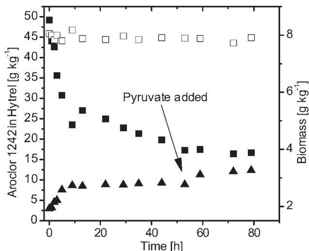
**Figure 5.** Biodegradation of Aroclor<sup>®</sup> 1242 by *B. xenovorans* LB400 in a solid-liquid TPPB. The filled squares show the PCB concentration in Hytrel<sup>™</sup> beads during biodegradation and the empty squares show the PCB concentration during a control experiment with deactivated biomass. The triangles represent the biomass concentration during the biodegradation experiment.
