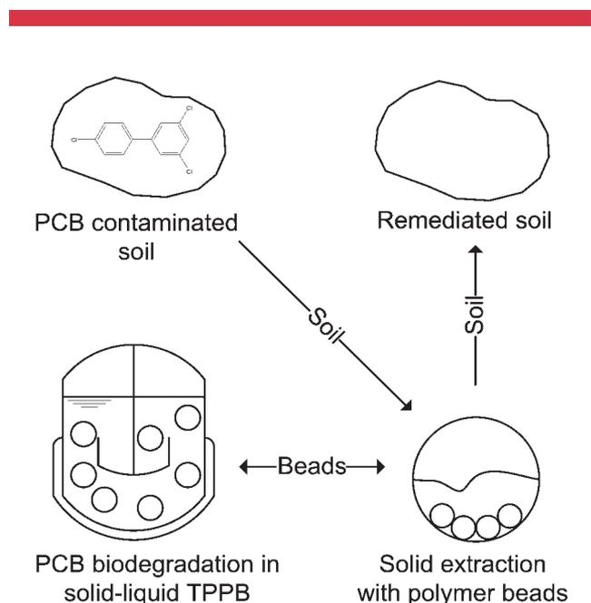
**Figure 1.** Schematic of soil remediation process. PCB contaminated soil is mixed with a solid extraction phase (polymeric material) in the presence of iso-propyl alcohol. PCBs are transferred from the soil to the polymers, the remediated soil is returned to the environment and the polymers are treated in a solid-liquid TPPB for microbial PCB destruction.
