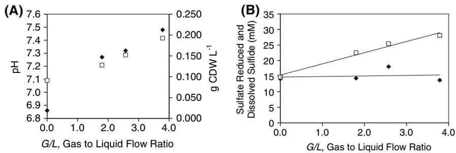
**Fig. 1** (a) (◆) pH and (□) suspended biomass concentration (g CDW L<sup>-1</sup>) as a function of  $G/L$  in a packed bed bioreactor ( $L = 80 \text{ ml h}^{-1}$ ). (b) (◆) Dissolved sulfide (mM) and (□) sulfate reduced (mM) as a function of  $G/L$  in a packed bed bioreactor. Samples were taken from the bioreactor's 3rd
