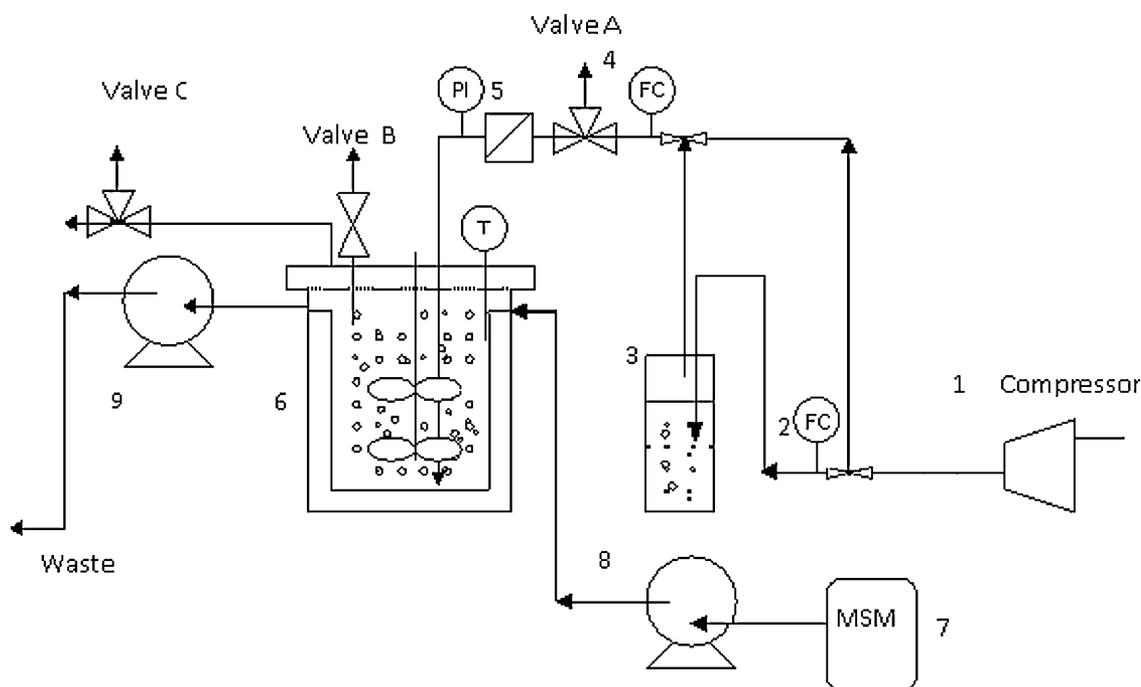
**Figure 1.** Schematic illustration of the experimental set-up. 1, Compressor; 2, Mass flow controller; 3, hexane evaporator; 4, mass flow controller; 5, air-filter; 6, stirred tank reactor; 7, MSM reservoir; 8, MSM influent pump; 9, waste effluent pump. PI, pressure indicator; T, temperature indicator; VALVE A, inlet gas phase sampling; VALVE B, liquid sampling; VALVE C, outlet gas phase sampling.
