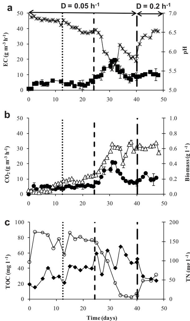
**Figure 4.** Time course of EC (■), pH (○),  $\text{CO}_2$  production rates (●), biomass concentration (Δ), TOC (◆), and TN (○) during hexane biodegradation by *P. aeruginosa* without a NAP (days 0–12), with Kraton G1657 (days 12–24) and with SO200 (day 24 and onwards). Vertical bars represent standard deviation.
