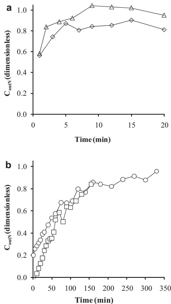
**Figure 2.** Time course of  $C_{outN}$  during the abiotic hexane mass transfer tests conducted in a fermentor without NAP (- $\Delta$ -) and with 20% of Kraton G1657 (- $\diamond$ -) (a) and with 20% of SO200 (- $\square$ -) and 20% of SO20 (- $\circ$ -) (b).
