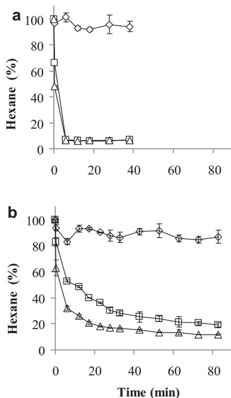
**Figure 3.** Time course of the hexane headspace concentration in the gas-tight tests carried out with SO200 (a) and KratonG1657 (b) as NAP. Diamonds, squares, and triangles represent systems supplied with MSM, MSM + NAP, and NAP, respectively. Vertical bars represent standard deviations.
