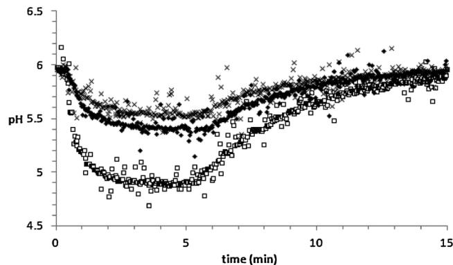
**Figure 3.** pH adjustment of modified Medium B containing varying amounts of butyric acid using  $\text{CO}_2\text{-N}_2$  sparging tests at atmospheric pressure. Crosses represent medium with  $10 \text{ g L}^{-1}$ , Closed diamonds represent medium with  $5 \text{ g L}^{-1}$  butyric acid, and open squares represent Medium B.
