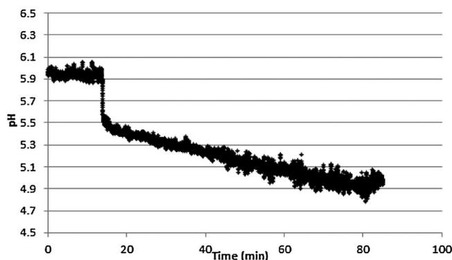
**Figure 5.** pH adjustment and subsequent butyric acid extraction from fermentation broth (*C. tyrobutyricum*) after 12 h using CO<sub>2</sub>-N<sub>2</sub> sparging at atmospheric pressure.
