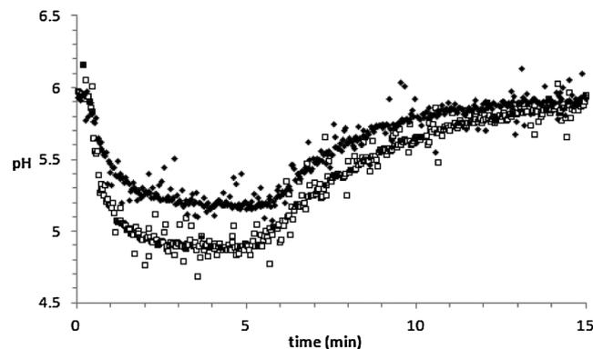
**Figure 2.** pH adjustment of media tested using  $\text{CO}_2\text{-N}_2$  sparging tests at atmospheric pressure. Closed diamonds represent an original Medium A, and open squares represent improved pH swingable Medium B.
