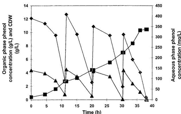
**Figure 3.** Time-course plot of organic-phase phenol (▲), aqueous-phase phenol concentration (◆), and cell dry weight (■) during fermentation with AVP2 as the catalyst and Adol 85 NF as the solvent phase in a 1:1 phase ratio.
