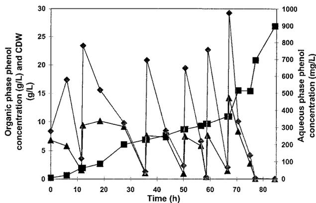
**Figure 4.** Time-course plot of organic-phase phenol (▲), aqueous-phase phenol concentration (◆), and cell dry weight (■) during extended fed-batch fermentation with 11172 as the catalyst and decanol as the solvent phase in a 3:1 (aqueous:solvent) phase ratio.
