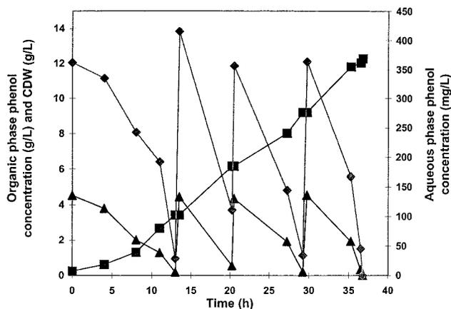
**Figure 2.** Time-course plot of organic-phase phenol (▲), aqueous-phase phenol concentration (◆), and cell dry weight (■) during fermentation with *P. putida* ATCC 11172 as the catalyst and Adol 85 NF as the solvent phase in a 1:1 phase ratio.
