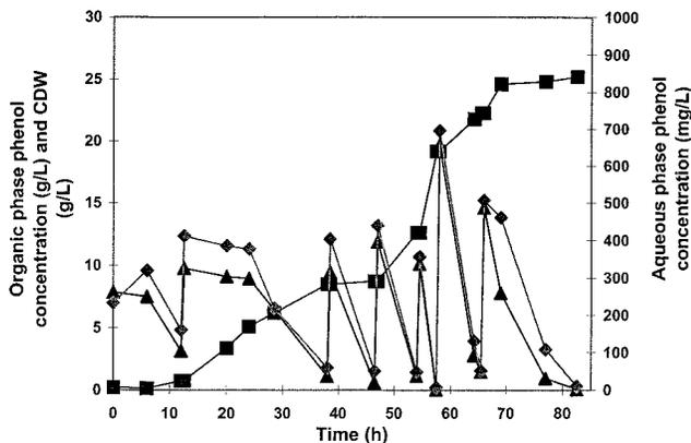
**Figure 5.** Time-course plot of organic-phase phenol (▲), aqueous-phase phenol concentration (◆), and cell dry weight (■) during extended fed-batch fermentation with AVP2 as the catalyst and decanol as the solvent phase in a 3:1 (aqueous:solvent) phase ratio.
