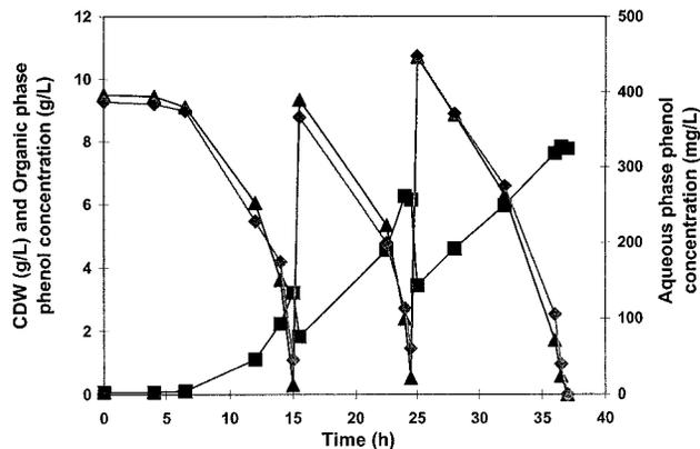
**Figure 6.** Time-course plot of organic-phase phenol (▲), aqueous-phase phenol concentration (◆), and cell dry weight (■) during cyclic-batch fermentation with AVP2 as the catalyst and decanol as the solvent phase in a 3:1 (aqueous:solvent) phase ratio.
