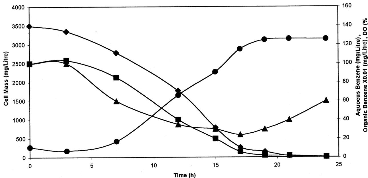
Fig. 3. Batch benzene degradation in the two-phase partitioning bioreactor with a condenser installed and with pure oxygen aeration. ●: cell mass, ■: benzene concentration in aqueous phase, ▲: DO level, ◆: benzene concentration in organic phase.
