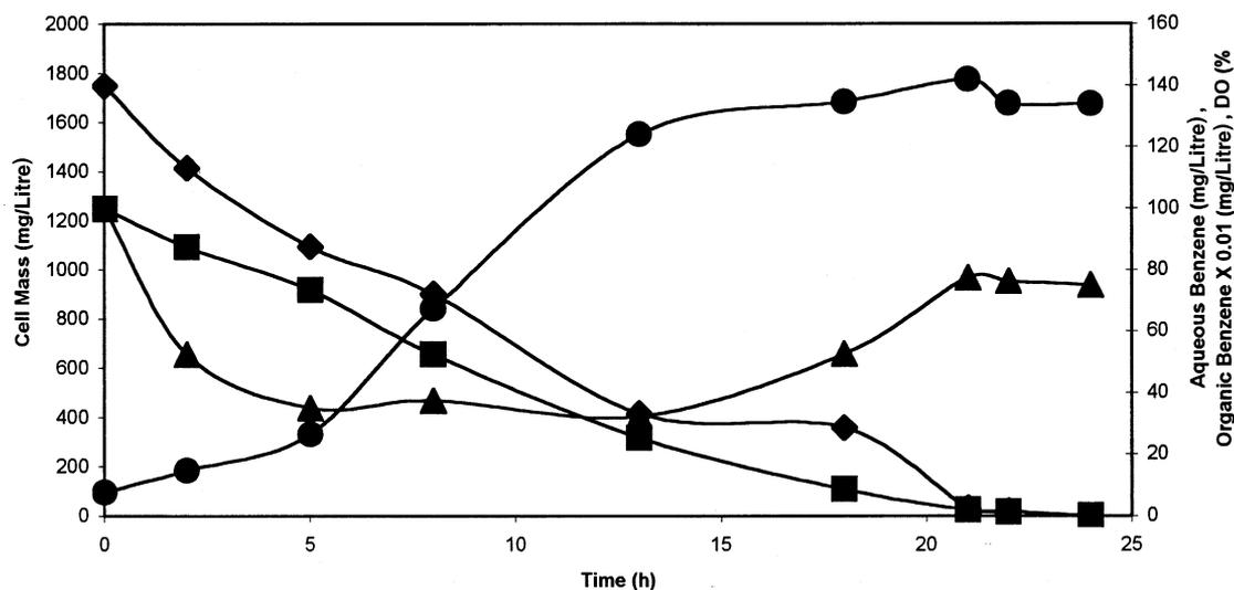
Fig. 1. Batch benzene degradation in the two-phase partitioning bioreactor. ●: cell mass, ■: benzene concentration in aqueous phase, ▲: DO level, ◆: benzene concentration in organic phase.
