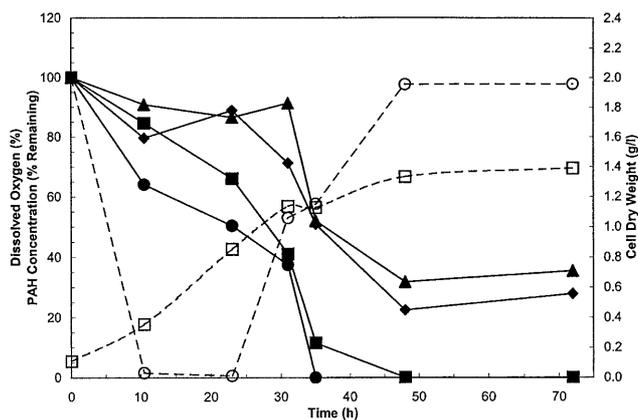
**Fig. 4** Degradation of four PAHs using a TPPB with a dodecane solvent phase. Changes in the organic phase naphthalene (*closed circles*), phenanthrene (*closed squares*), anthracene (*closed diamonds*) and acenaphthene (*closed triangles*) concentrations, and in aqueous cell dry weight (*open squares*) and % dissolved oxygen (*open circles*) in the fermentor are shown
