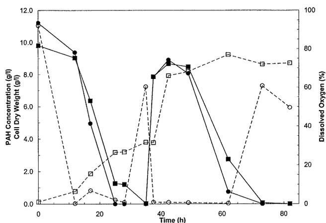
**Fig. 6** Degradation of a high concentration of PAHs in a TPPB using a sequential feeding strategy. Changes in the organic phase naphthalene (closed circles) and phenanthrene (closed squares) concentrations, and in aqueous cell dry weight (open squares) and % dissolved oxygen (open circles) in the fermentor are shown
