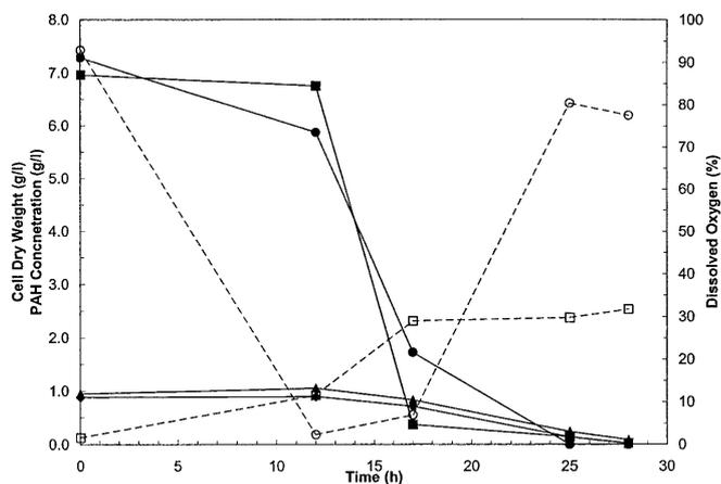
**Fig. 5** Complete degradation of four PAHs in a TPPB using new nutrient conditions. Changes in the organic phase naphthalene (closed circles), phenanthrene (closed squares), anthracene (closed diamonds) and acenaphthene (closed triangles) concentrations and in cell dry weight (open squares) and % dissolved oxygen (open circles) in the fermentor are shown
