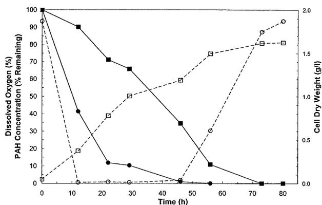
**Fig. 2** Proof of concept – degradation of two low molecular weight (LMW) PAHs in a two-phase partitioning bioreactor (TPPB). Changes in the organic phase naphthalene (*closed circles*) and phenanthrene (*closed squares*) concentrations, and in aqueous cell dry weight (*open squares*) and % dissolved oxygen (*open circles*) in the fermentor are shown
