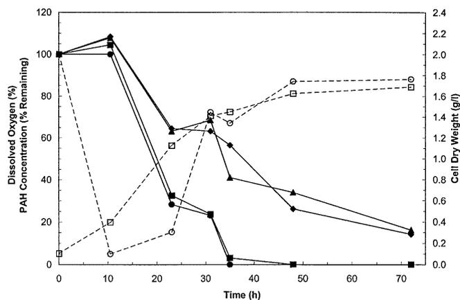
**Fig. 3** Degradation of four PAHs using a TPPB with a dodecane/ethanol solvent phase. Changes in the organic phase naphthalene (*closed circles*), phenanthrene (*closed squares*), anthracene (*closed diamonds*) and acenaphthene (*closed triangles*) concentrations, and in aqueous cell dry weight (*open squares*) and % dissolved oxygen (*open circles*) in the fermentor are shown
