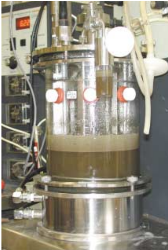
Fig. 2. A 5 l TPPB system degrading polyaromatic hydrocarbons (PAHs), in which multi-gram quantities of PAHs are dissolved in the organic phase, delivering milligram quantities to the cells in the aqueous phase. The solvent phase is dodecane and the organism is Sphingomonas sp.
